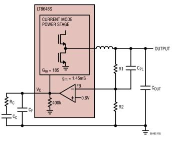
Figure 5. Model for Loop Response
