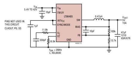
Figure 12. 2MHz 5V, 15A Step-Down Converter with Spread Spectrum
