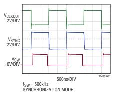
Switching Waveforms, Full Frequency Continuous Operation
