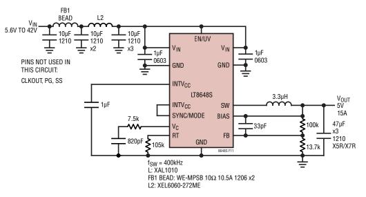
Figure 11. Ultralow EMI 5V, 15A Step-Down Converter with Spread Spectrum
