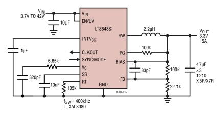
Figure 10. 400kHz 3.3V, 15A Step-Down Converter with Soft-Start and Power Good
