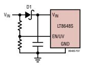
Figure 7. Reverse V<sub>IN</sub> Protection
