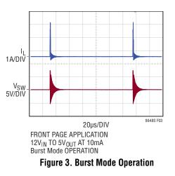
The output load at which the LT8648S reaches the programmed frequency varies based on input voltage, output voltage and inductor choice. To select low ripple Burst Mode operation, tie the SYNC/MODE pin below 0.7V (this can be ground or a logic low output).
