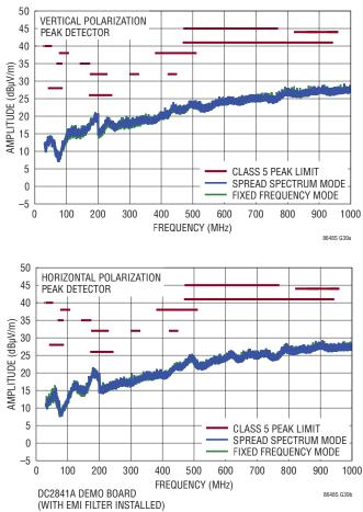
(WITH EMI FILTER INSTALLED) 14V INPUT TO 5V OUTPUT AT 15A, f<sub>SW</sub> = 400kHz
