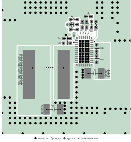
Figure 1. Recommended PCB Layout
