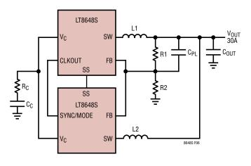
Figure 6. Paralleling Two LT8648Ss
